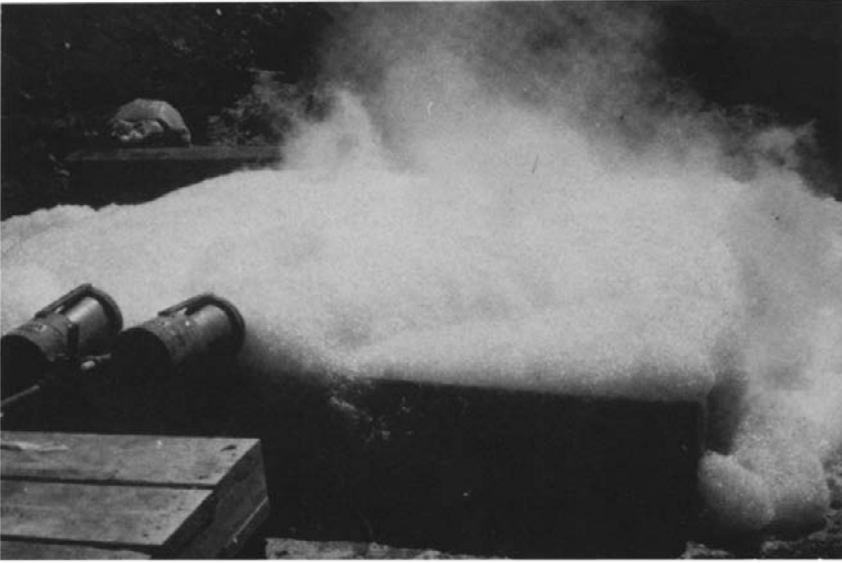
Fig. 2. Vapor release through foam blanket using ammoniated foam.
