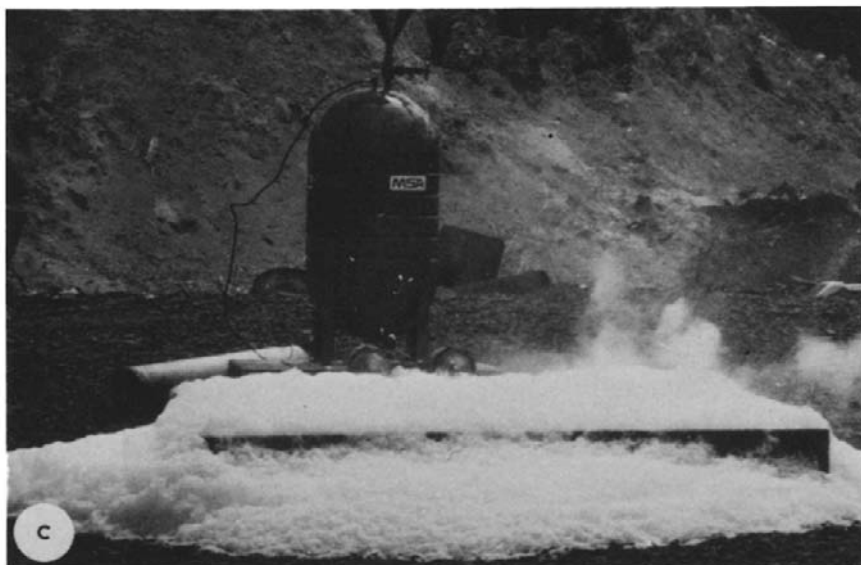
Fig. 1. Spill sequence for foam—silicon tetrachloride test. (a) Free spill; (b) foam on; (c) foam blanket in place.
